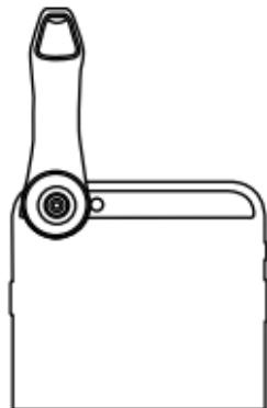
2. Make sure the clamp is directly over the camera of the phone.
