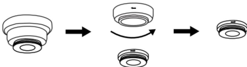
1. Fix and hold the top lens with one hand.
