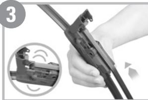
4 With wiper arm securely inserted into the adapter, close adapter cover.
