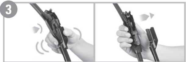
With wiper arm securely inserted into the adapter, close adapter cover.
