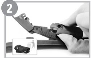
3 Pull blade upwards to secure the wiper arm into the adapter as shown.
