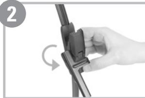
3 Ensure that wiper blade is secured on the wiper arm.
