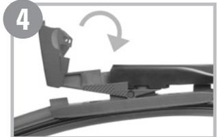
5 An audible "click" must be heard to ensure that blade is secured on the wiper arm.
