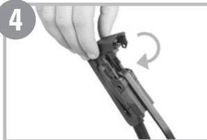
5 An audible "click" must be heard to ensure that blade is secured on the wiper arm.
