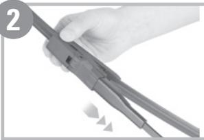
An audible "click" must be heard to ensure that blade is secured on the wiper arm.
