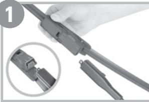
Insert blade into adapter opening as shown.
