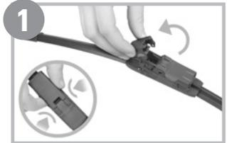
2 Peel and remove the adapter piece as shown.
