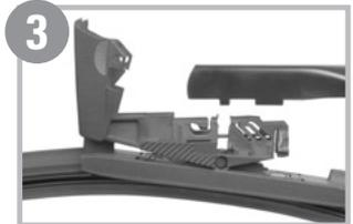
4 With wiper arm securely inserted into the adapter, close adapter cover.
