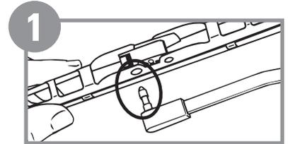
Align wiper arm with wiper blade pin hole as shown.
