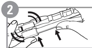
Insert wiper arm into the wiper blade pin hole.
