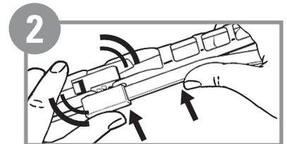
Insert wiper arm into the wiper blade pin hole.
