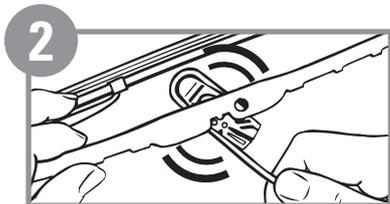
Pull blade upwards to secure the wiper arm into the adapter.
