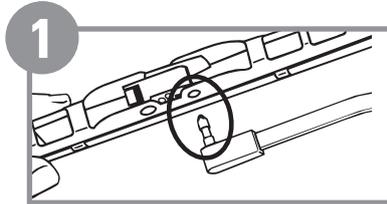
Align wiper arm with wiper blade pin hole as shown.
