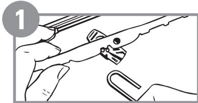
Rotate wiper adapter and insert hook arm as shown.
