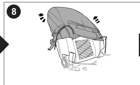
Install new pad, peel & stick adhesive. Note: Be sure to route wiring to bottom of seat back, away from center of the seat.
