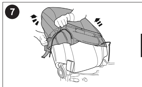
Remove seat back cover, and remove old heating pad (if so equipped). Note: Slide cover up only as far as needed to install seat heater pad.
