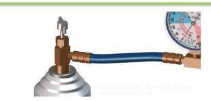
2. Screw can tap end of the installation hose onto RED TEK can.
