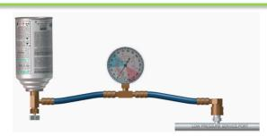
4. With engine off, turn can upside down and turn the can tap handle clockwise until the piercing needle opens the self-sealing valve on the RED TEK
