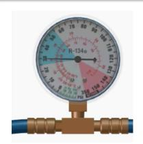
5. After minimum charge (30psi) is achieved, start the vehicle and turn A/C system to highest setting. Make sure compressor is engaged/functioning.
