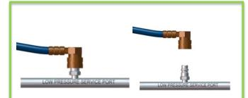
7. Remove quick coupler by pulling sleeve up.
