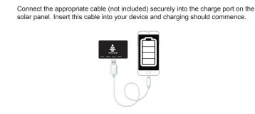
For the DC port, ensure the correct cable is used. Check with the manufacturer of the device intended to charge to ensure it can be used with a solar panel and choose a compatible cable.
