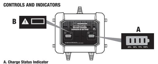
This battery charger has an easy-to-follow 4-LED charge status indicator: 25%, 50%, 75%, 100%. This indicator provides an estimate of the battery's state of charge as charging progresses. During charging, the corresponding state of charge LED will be flashing. When the 100% LED lights solid (i.e., stops flashing), the battery is fully charged and the charger has entered the Maintain stage (see Understanding the Multi-stage Charging Process).
