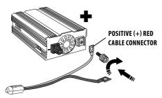
Place the black cable connector on the negative DC cabling terminal (- / black). Make sure that the
