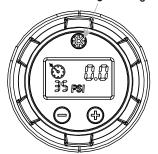
When the inflator is turned on, the flashlight can be powered on or off manually by pressing the button (see illustration); if the inflator is not activated after 30 seconds of powering on, the flashlight will automatically turn off.
