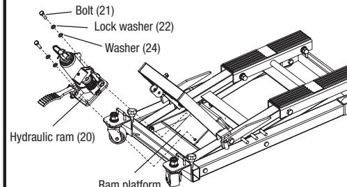
**2** Attach Hydraulic Ram & Lock Bar
